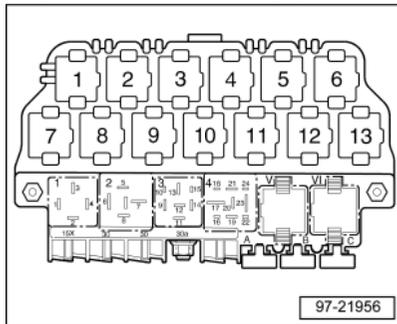
Relay locations on the 8 position additional relay carrier
